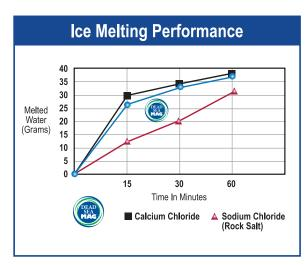
The tests were performed by the Swedish VTI by spreading 10 grams of each ice melter evenly over an icy surface at +21°F.
